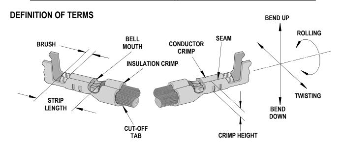
The above terminal drawing is a generic terminal representation. It is not an image of any terminal listed in the scope.
