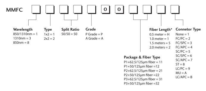
$<sup>^*</sup>$  The tolerance of fiber length is +/-0.1m. 1 meter is standard. The lead time for special fiber length will be longer.
