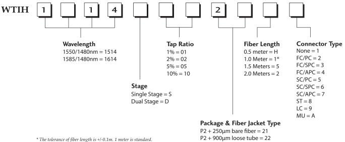
\* The tolerance of fiber length is +/-0.1m. 1 meter is standard. The lead-time for special fiber length will be longer.
