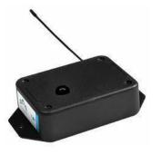
The wireless motion detection sensor uses an infrared sensor to accurately detect movements made by people, animals or other things within 16.4 ft (5 m) range. Up to 10-Year Battery Life
