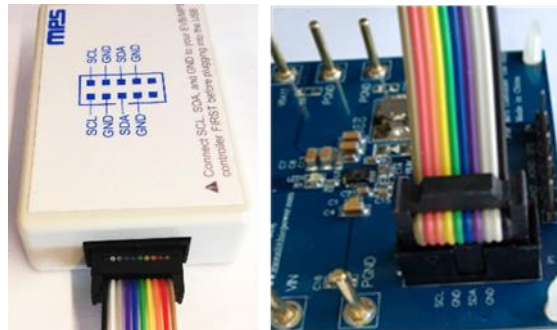
Figure 6: EVB to MPS I 2 C Communication Interface Wire Connection
