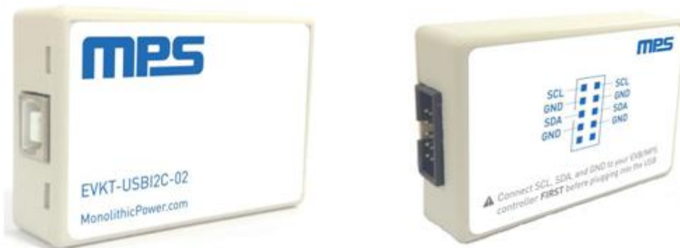
Figure 3: EVKT-USBI2C-02 Communication Interface
