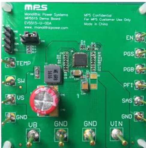
Figure 2: EV5515-U-00A Evaluation Board
