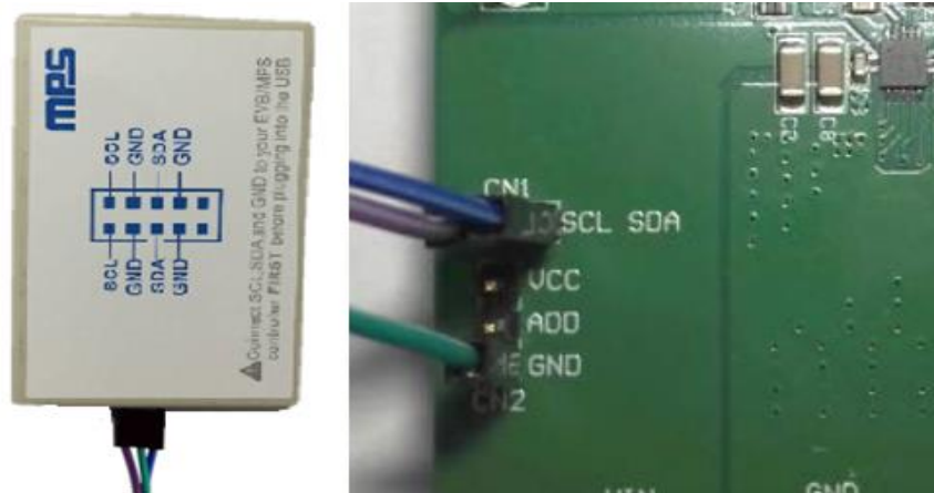
Figure 6: EVB to MPS I 2 C Communication Interface Wire Connection
