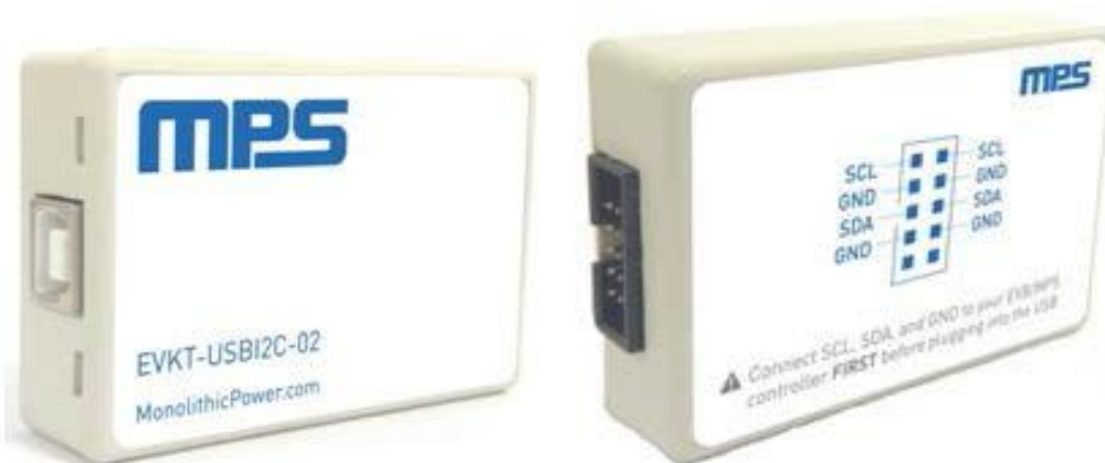
Figure 3: EVKT-USBI2C-02 Communication Interface
