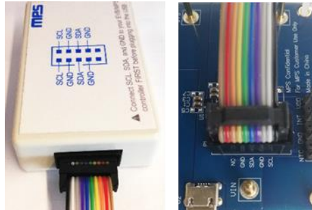
Figure 6: EVB to MPS I 2 C Communication Interface Wire Connection
