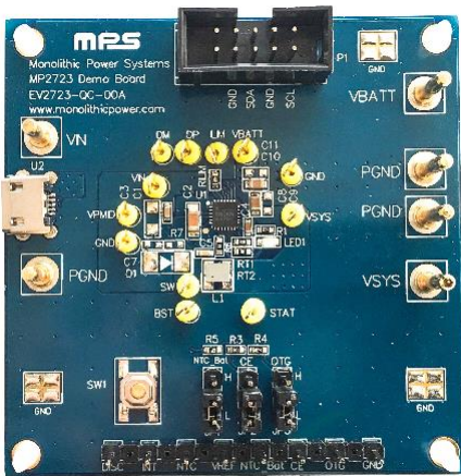
Figure 2: EV2723-QC-00A Evaluation Board
