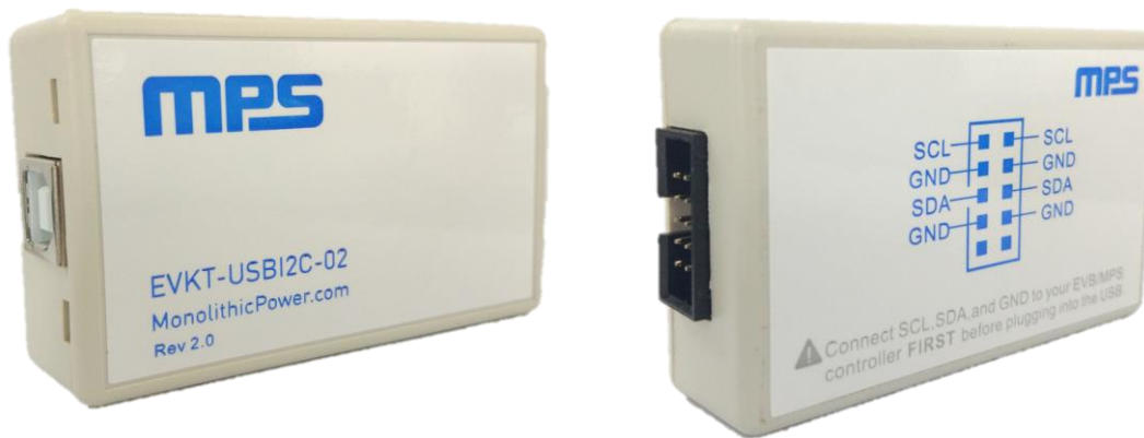
Figure 3: EVKT-USBI2C-02 Communication Interface
