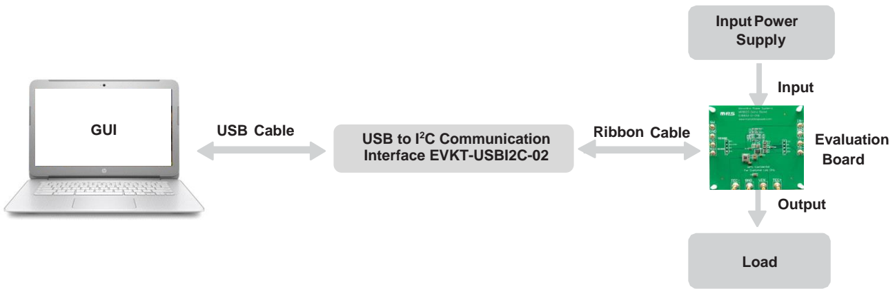
Figure 1: EVKT-MP8833 Evaluation Kit Set-Up
