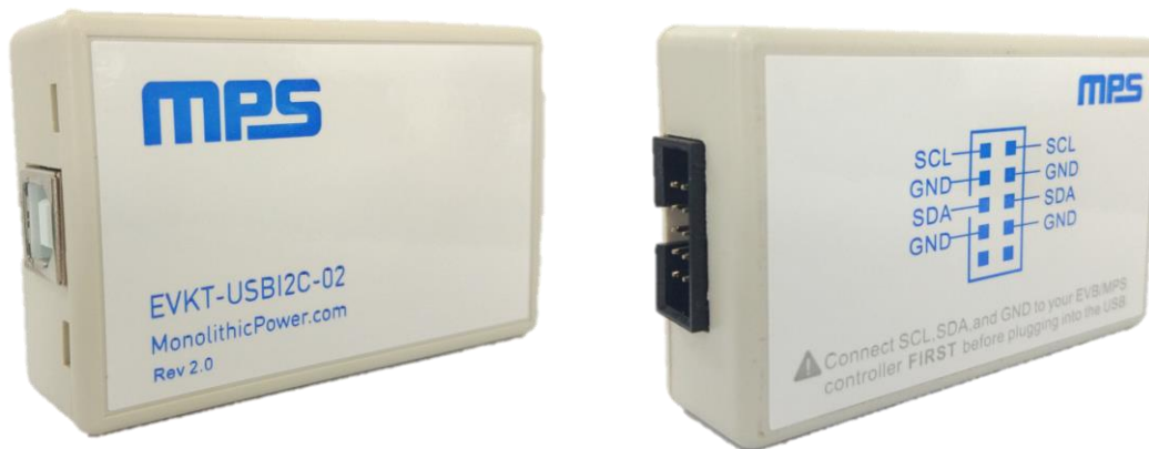
Figure 3: EVKT-USBI2C-02 Communication Interface Device
