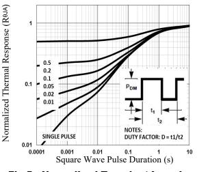
Fig.5 Normalized Transient Impedance
