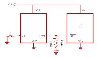
Detector output remains low if V<sub>IN</sub>is below detecting level, and jumps to high if VIN is above detecting level for 240ms
