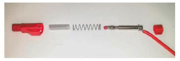
Note: Use very short wire strip length and solder just above the spring retainer.
