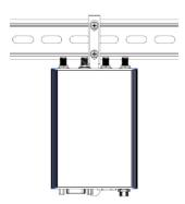
**Notes:** 1) Package contents include DIN Rail clips and associated hardware for mounting devices in the orientation shown above. 2) Clips onto 35mm and 32mm DIN rails.
