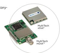
The mDot and xDot are LoRaWAN compliant,
