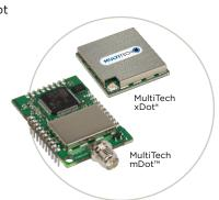
The mDot and xDot are LoRaWAN compliant,
