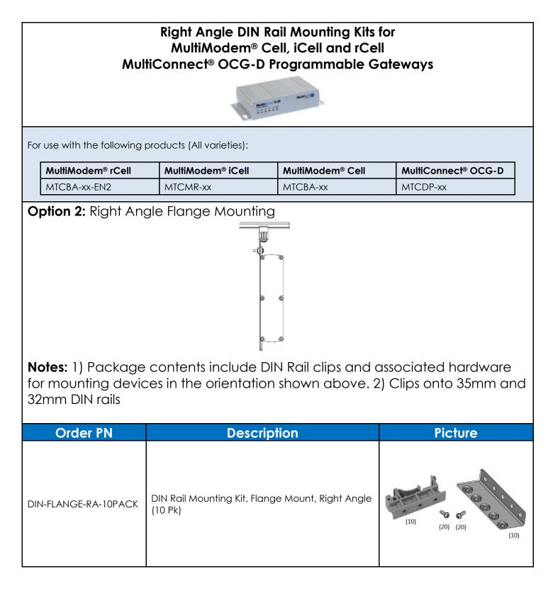
Note: DIN rail support is available now on all MultiConnect® rCell 100 and Cell 100 series products.
