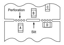
\*1 A > D is valid when stress is added vertically to the perforation as with Hand Separation. If a Cutting Disc is used, stress will be diagonal to the PCB, therefore A > D is invalid.
