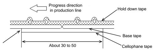
No lifting for the direction of progressing
