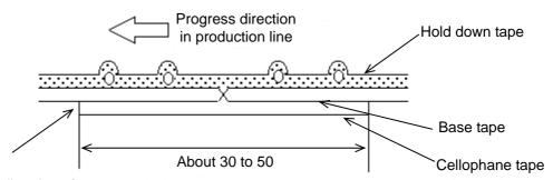
No lifting for the direction of progressing
