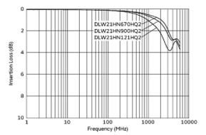
Differential Mode Transmission Characteristics (Typical Value)
