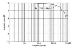
Differential Mode Transmission Characteristics (Typical Value)
