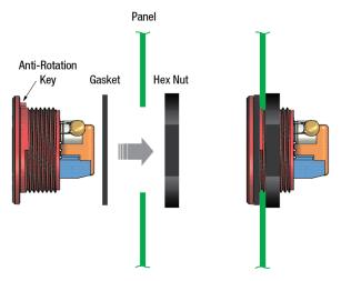
Figure 1. Panel Installation
