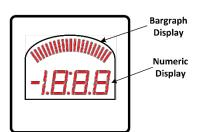
**Bar-graph Display:** The 21 segment bar-graph display responds quickly and smoothly like an analog meter movement to aid in reading rapidly changing measurements.
