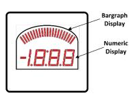
**Bar-graph Display:** The 21 segment bar-graph display responds quickly and smoothly like an analog meter movement to aid in reading rapidly changing measurements.
