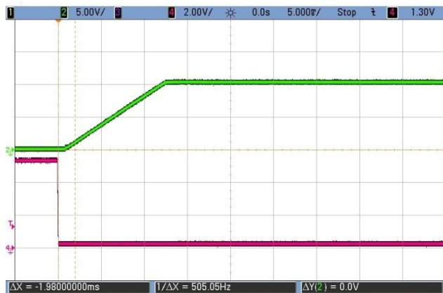
Turn-on transient at full load current (5ms/div, Top Trace: V out , 5V/div; Bottom Trace: ON/OFF, 2V/div)
