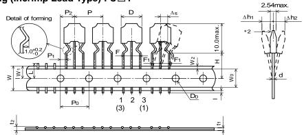
\*1.Bottom of dielectric may be exposed.\*2.There should not be the exposure of the ferrite bead if a hole is on the top of ferrite bead.
