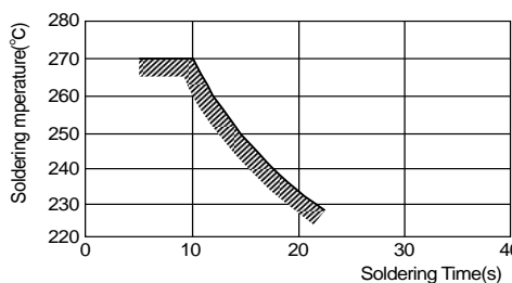
[Allowable Flow Soldering Temperature and Time]
