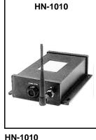
The HN-1010 is enclosed in a NEMA 4X and I.P. 66 rated housing and can operate outdoors from -30OC to +70OC. The unit features a 9 pin I/O connector for data, power, and flow control. Transmit and receive data are RS-485 compatible differential signals while the flow control lines are single-ended RS-232. This interface can drive up to 250 feet of cable and can be converted to plain RS-232 using the HopNet 3500 data/power adapter.
