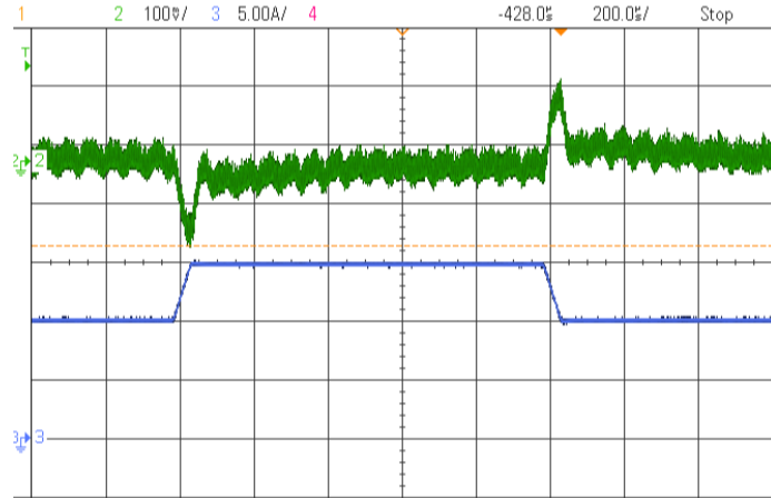
Output voltage response to step-change in load current Vin=72V (50%-75%-50% of full load; di/dt = 0.1A/μs). Trace: Vout: 100mV/div; Iout: 5A/div; Time: 200us/div
