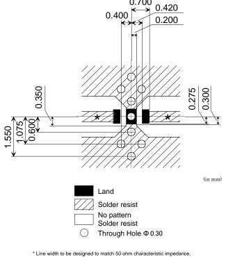
\* Line width to be designed to match 50 ohm characteristic impedance, Depending on PCB material and thickness.
