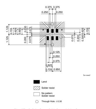
\*Line width to be designed to match  $50\Omega$  characteristic impedance, depending on PCB material and thickness.
