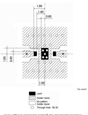
$^{\star}$  Line width to be designed to match 75 ohm characteristic impedance,  $Depending \ on \ PCB \ material \ and \ thickness.$
