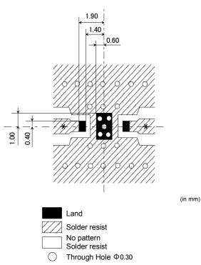
\* Line width to be designed to match 75 ohm characteristic impedance, Depending on PCB material and thickness.
