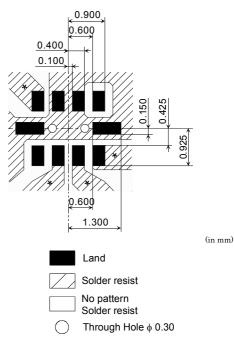
\*Line width to be designed to match 50\Omega characteristic impedance, depending on PCB material and thickness.
