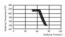
In case of repeated soldering, the accumulated soldering time must be within the range shown above.
