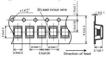
%The packing directions of the chip coil in taping are unified with the in/out positions of the lead wire.
