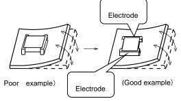
Products shall be located in the sideways direction (Length:a<b) to the mechanical stress.
