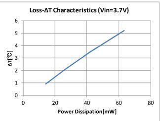
The output current of the device may need to be de-rated if it is operated in a high ambient temperature or in a continuous power delivering application. The amount of current de-rating is highly dependent on the environmental thermal conditions, i.e. PCB design, nearby components or effective air flows. Care should especially be taken in applications where the device temperature exceeds 85°C.
