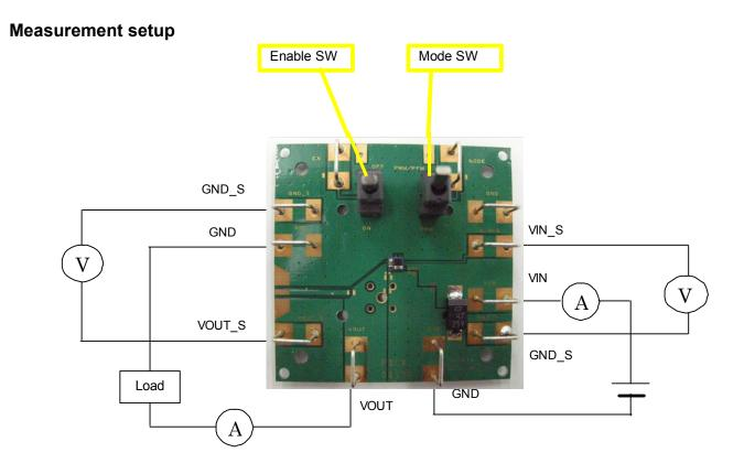
The enable switch has three positions.
