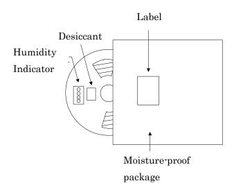
Reel will be packed in moisture-proof package together with desiccant and humidity indicator. After packing, the package will be heat-sealed.
