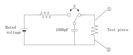
Fig 2 Applied voltage
