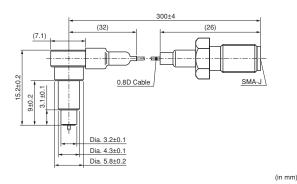
Measurement Probe for MM8030-2610 (P/N: MXHQ87WJ3000)
