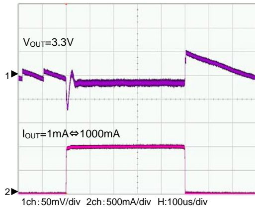
MYRGM330150B31RA ( V_{IN}=5V , I_{OUT}=1mA \leftrightarrow 1000mA )
