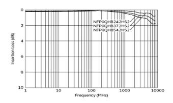
Common Mode Insertion Loss Characteristic (Typical Value)
