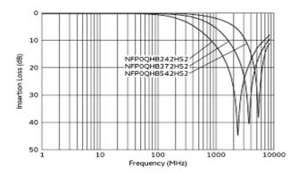
**Differential Mode Transmission Characteristics** (Typical Value)
