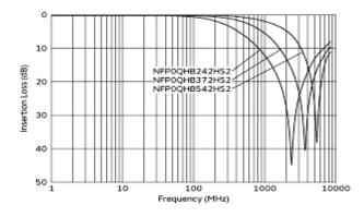
**Differential Mode Transmission Characteristics** (Typical Value)
