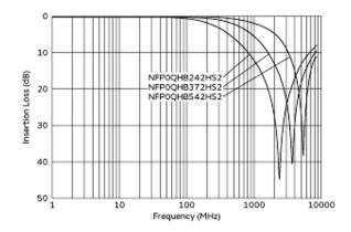
Common Mode Insertion Loss Characteristic (Main Items)(Typical Value)
