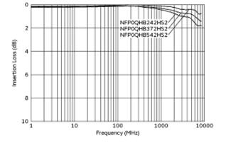
Common Mode Insertion Loss Characteristic (Typical Value)
