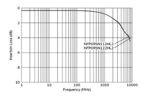
Common Mode Insertion Loss Characteristic (Typical Value)
